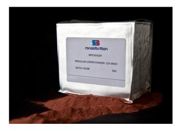
Vacuum packing is particularly useful if the powder is to be used in small quantities at a time. Typically, if a 25kg drum of powder is opened several times before consumption, the exposure to air/humidity at each lid opening can adversely affect powder shelf-life. This can be detrimental to applications where excessive powder oxidation reduces performance or product appearance.
