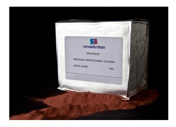
Vacuum packing is particularly useful if the powder is to be used in small quantities at a time. Typically, if a 25kg drum of powder is opened several times before consumption, the exposure to air/humidity at each lid opening can adversely affect powder shelf-life. This can be detrimental to applications where excessive powder oxidation reduces performance or product appearance.
